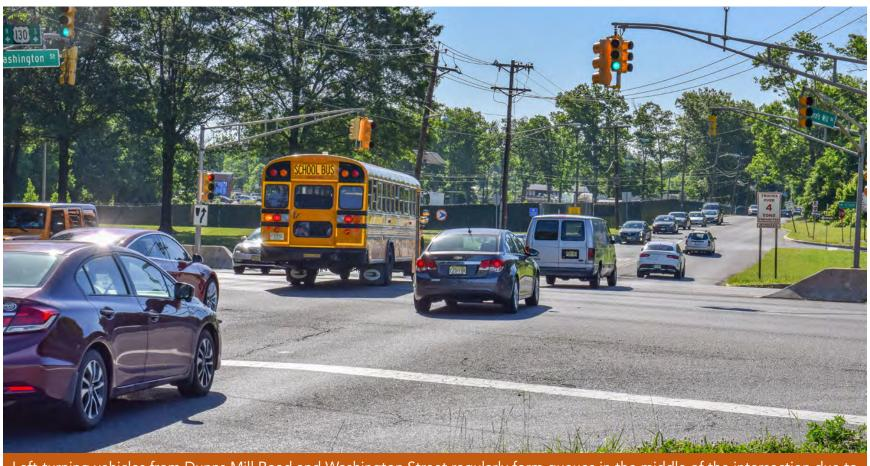
Left-turning vehicles from Dunns Mill Road and Washington Street regularly form queues in the middle of the intersection due to poor visibility of through-traffic
